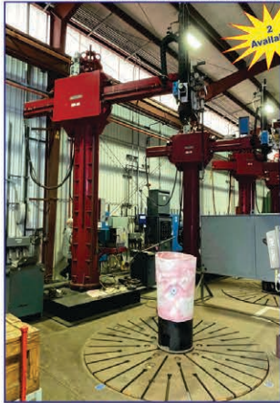
Clad Unit #1: A&N Plant Model RC40X3.75 Cladding Machine with Arc Specialties Hot One Solid State Hotwire Power Supply and Esab 350 MPI MIG Welder
