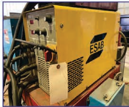
Clad Unit #1: A&N Plant Model RC40X3.75 Cladding Machine with Arc Specialties Hot One Solid State Hotwire Power Supply and Esab 350 MPI MIG Welder
